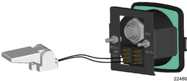
High-Water Float Switch Connection to Operator Module
